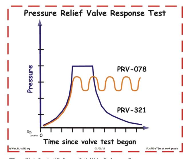
sTEm-at-Work (Puzzle #17): Pressure Relief Valve Performance Test
